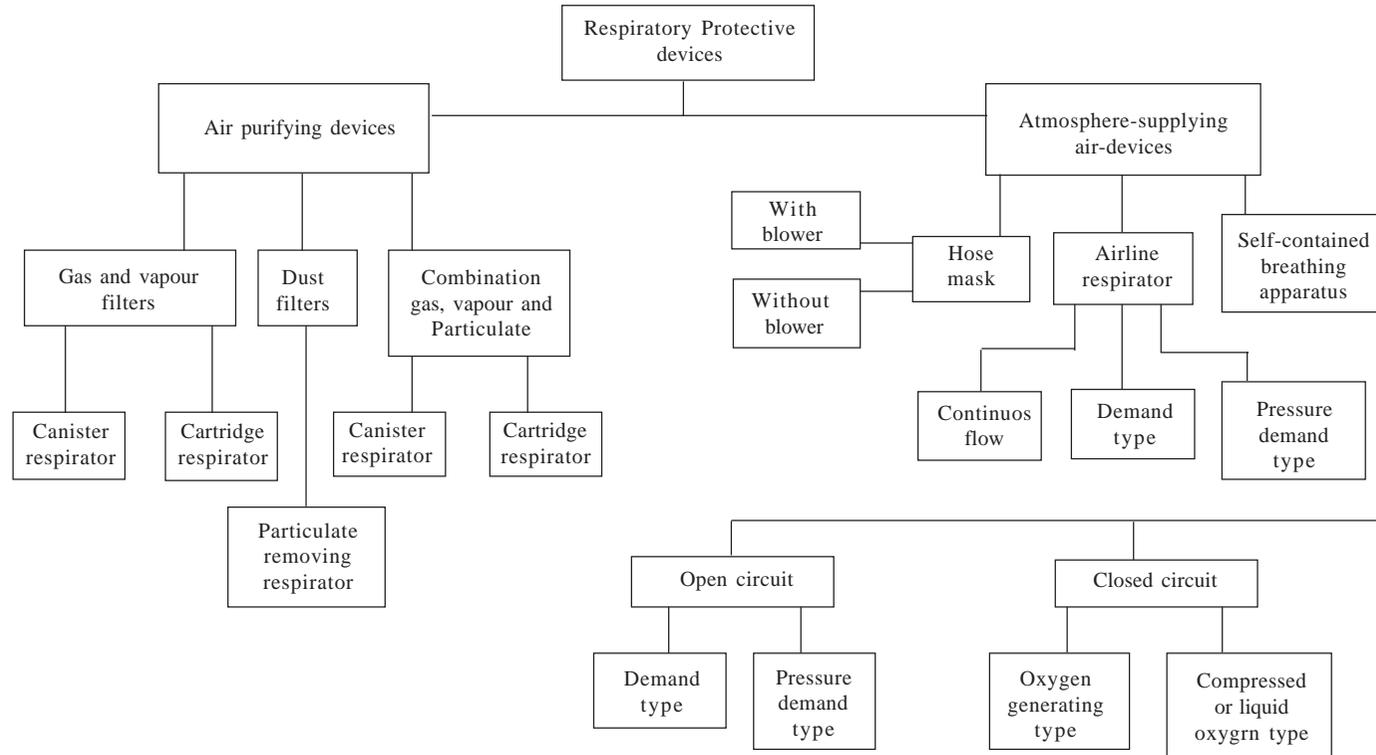
**FIGURE 3: ENVIRONMENT CLASSIFICATION FOR SELECTION OF RESPIRATORY PROTECTION DEVICES**
